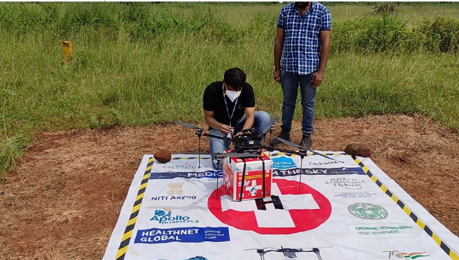
FIGURE 17c | Vaccine-loaded payload box being mounted on a drone for a BVLOS flight
