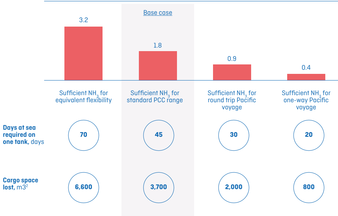
Exhibit 26: Cargo capacity loss for dual-fuel PCC carriers under different ammonia fuel tank assumptions
