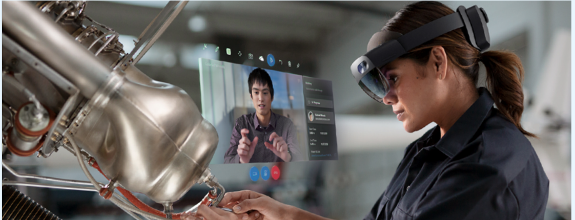
FIGURE 7 AR for enabling remote expert collaboration
