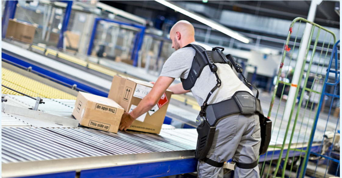
FIGURE 4 Exoskeletons helping operators in logistics
